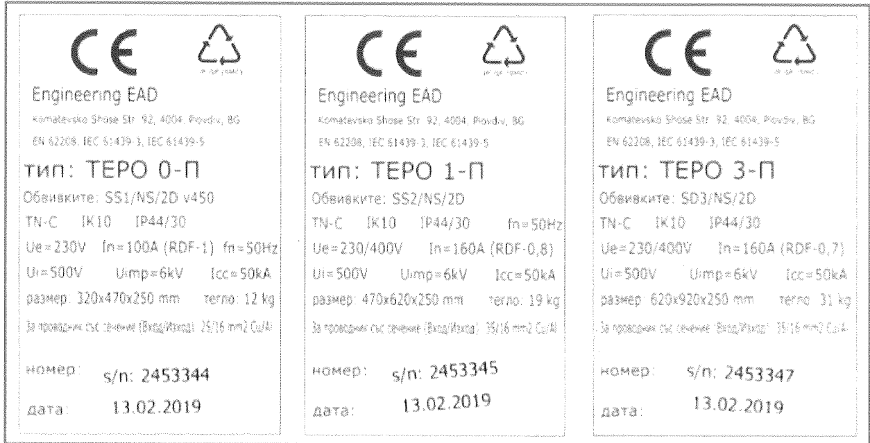
Fig. 1 – Labels of switchgears
